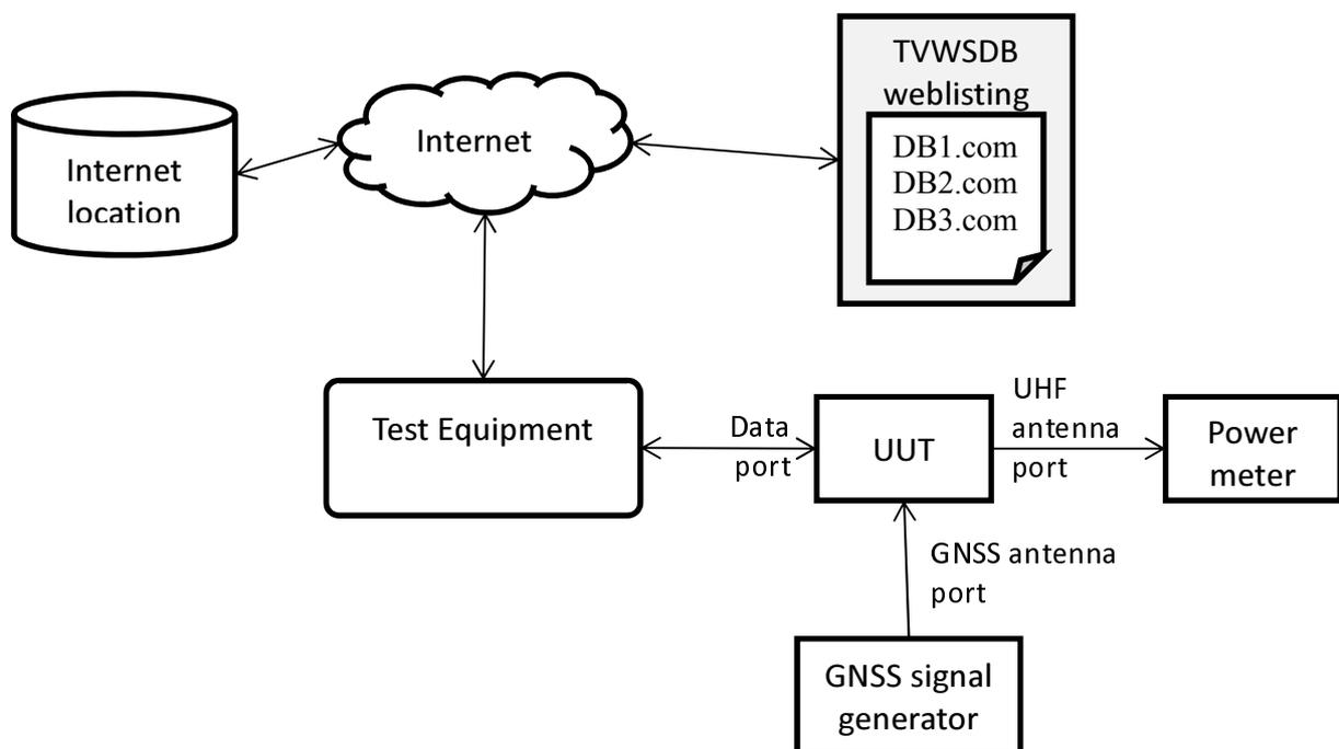
**Figure 4a: Test arrangement for test database identification and access**
