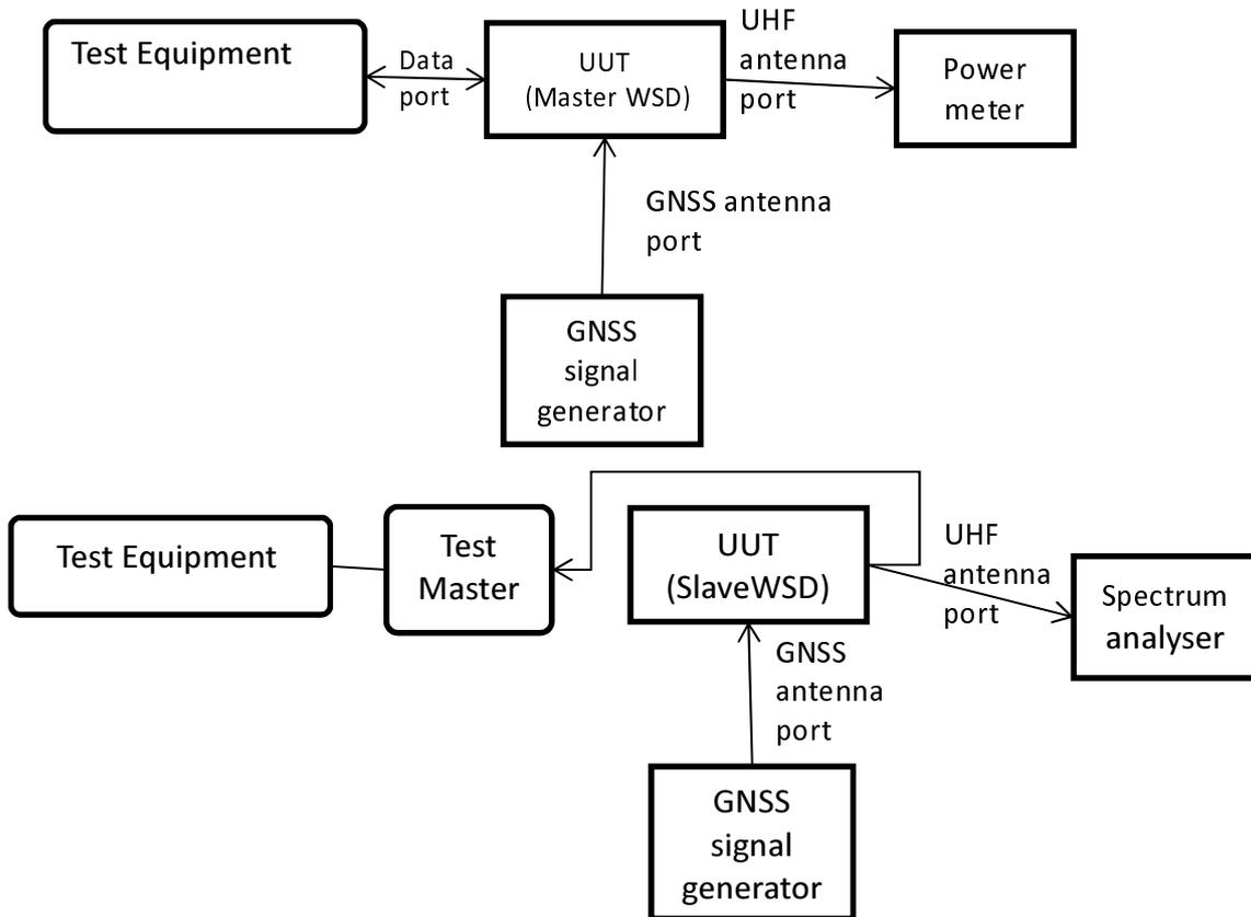
**Figure 5: Test arrangement for Geo-location capability**
